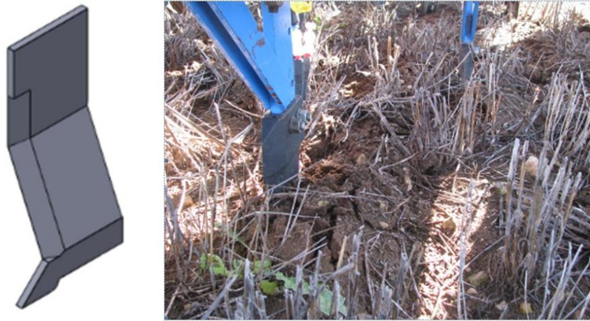
Figure 2. Bent leg furrow opener (left) with offset soil disturbance pattern in the field (right).
